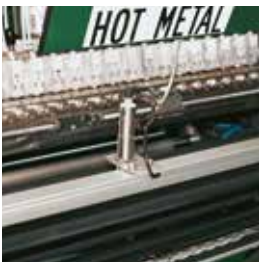
Winding diameter measuring at the laminating machine
