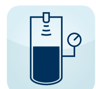
Monitoring filling level in 6 bar overpressure
